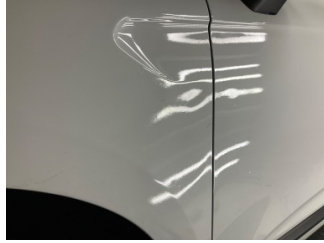
Çamurluk, sol, Çamurluk, sol > Ezik
