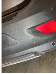
Tampon, arka, Arka tampon > Vuruk
