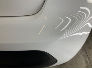
Tampon, arka, Arka tampon > Vuruk
