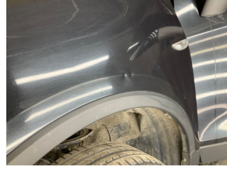
Çamurluk, sol, Çamurluk, sol > Ezik
