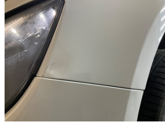
Çamurluk, sol, Çamurluk, sol > Ezik
