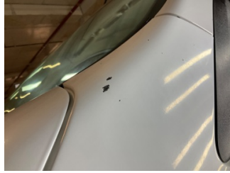
Çamurluk, sol, Çamurluk, sol > Ezik
