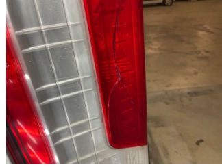
Arka lambalar, Arka lambalar, sol > Hasarlı
