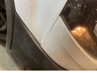
Çamurluk, sol, Çamurluk, sol > Ezik
