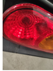
Arka lambalar, Arka lambalar, sol > Çatlak
