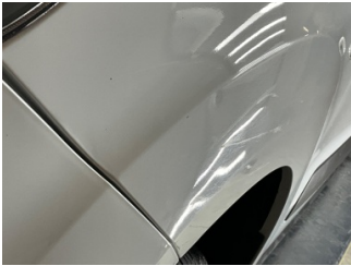
Çamurluk, sol, Çamurluk, sol > Ezik
