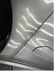
Çamurluk, sol, Çamurluk, sol > Ezik
