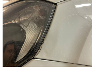
Çamurluk, sol, Çamurluk, sol > Ezik
