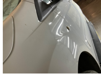
Çamurluk, sol, Çamurluk, sol > Ezik
