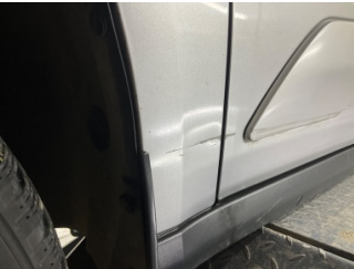
Çamurluk, sol, Çamurluk, sol > Ezik
