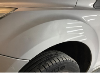
Çamurluk, sol, Çamurluk, sol > Ezik
