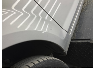
Çamurluk, sol, Çamurluk, sol > Ezik
