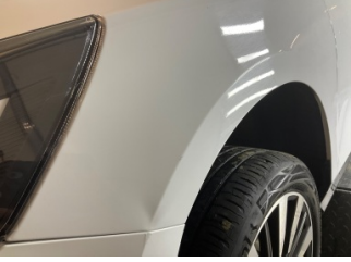
Çamurluk, sol, Çamurluk, sol > Ezik
