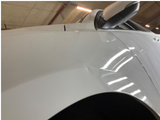
Çamurluk, sol, Çamurluk, sol > Ezik
