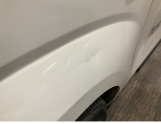
Çamurluk, sol, Çamurluk, sol > Ezik
