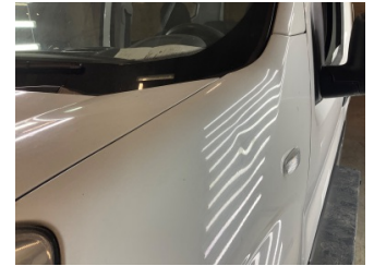
Çamurluk, sol, Çamurluk, sol > Ezik
