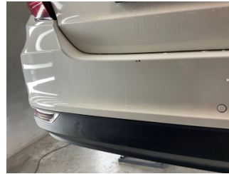
Tampon, arka, Arka tampon > Vuruk
