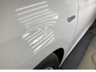
Çamurluk, sol, Çamurluk, sol > Ezik
