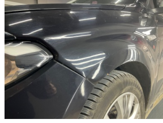
Çamurluk, sol, Çamurluk, sol > Ezik
