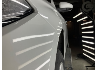
Çamurluk, sol, Çamurluk, sol > Ezik
