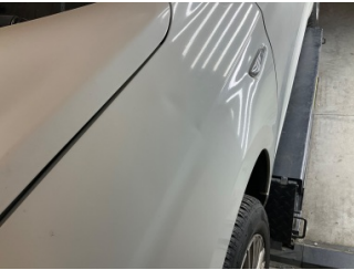
Çamurluk, sol, Çamurluk, sol > Ezik
