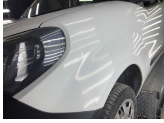
Çamurluk, sol, Çamurluk, sol > Ezik
