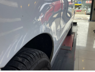
Çamurluk, sol, Çamurluk, sol > Ezik
