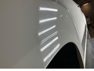
Çamurluk, sol, Çamurluk, sol > Ezik
