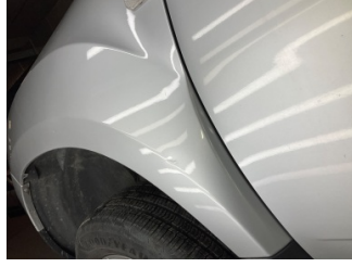
Çamurluk, sol, Çamurluk, sol > Ezik
