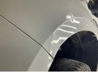
Çamurluk, sol, Çamurluk, sol > Ezik
