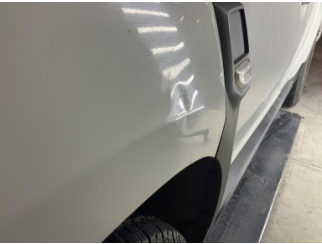
Çamurluk, sol, Çamurluk, sol > Ezik
