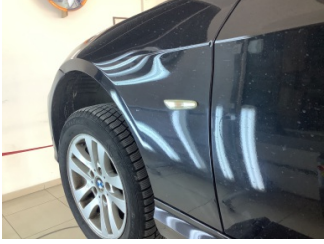
Çamurluk, sol, Çamurluk, sol > Ezik
